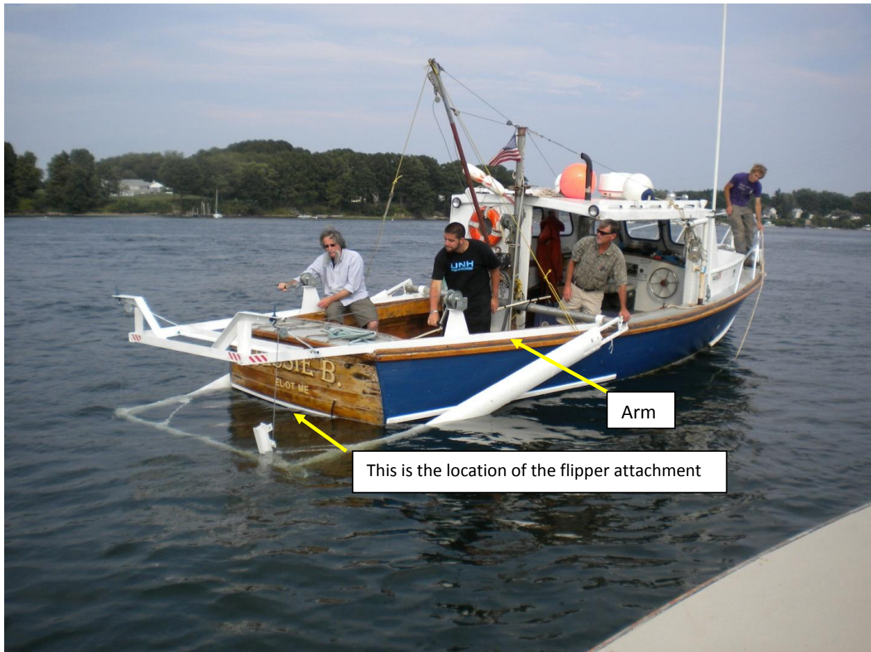
Figure 3. The flipper deployment frame mounted on the Jesse B . The flipper is lowered to a position under the vessel when the 'arms' are in a vertical position
