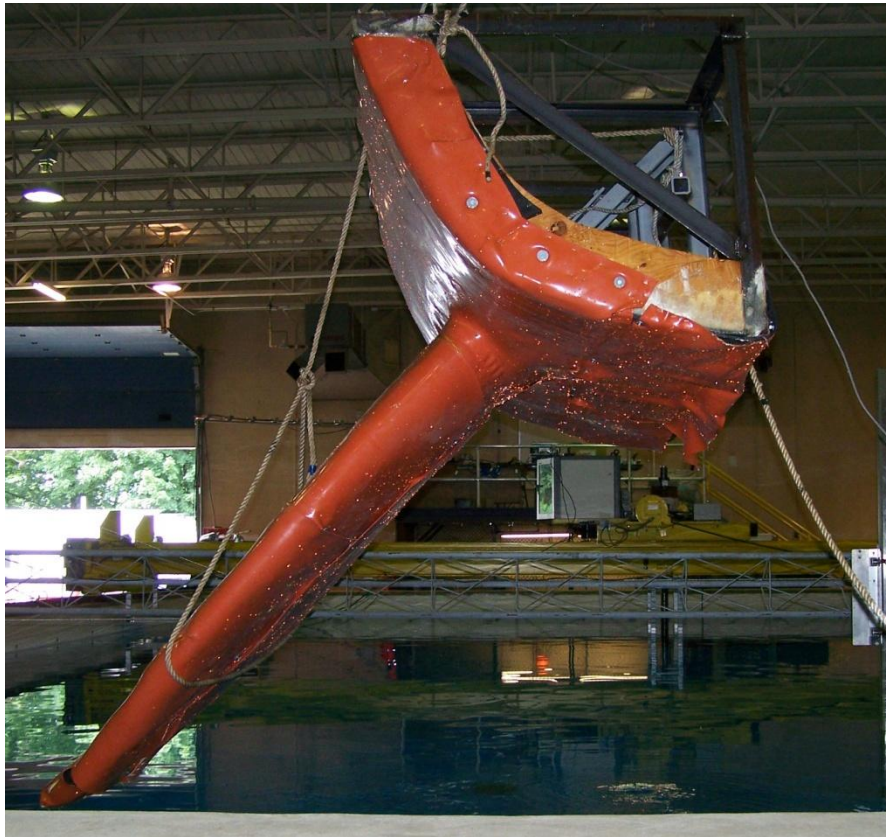
Figure 1. Completed flipper-whale body section while being weighed in air and water at UNH Chase Ocean Engineering Lab.
