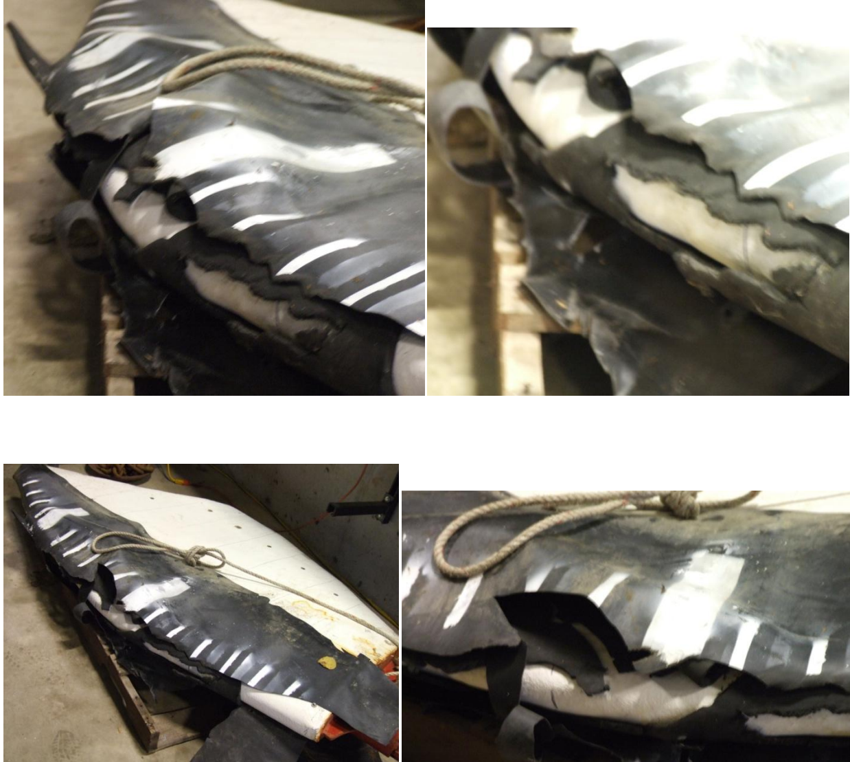
Figure 7. A series of after the fact pictures showing the status of the leading edge of the flipper. The top two pictures show a scalloped edge which is most likely resulting from a 'sawing action' of the line as the float descended.
