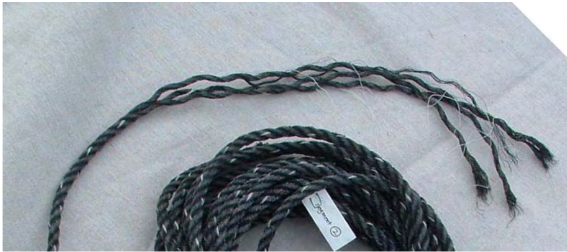
Frayed end may indicate tensile break
