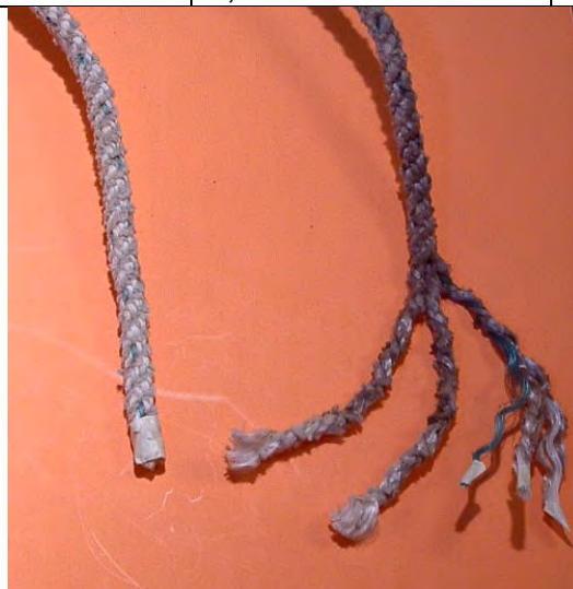
J031704 \frac{3}{8} 3-Strand PP/PET blend. Note uniform surface abrasion.
