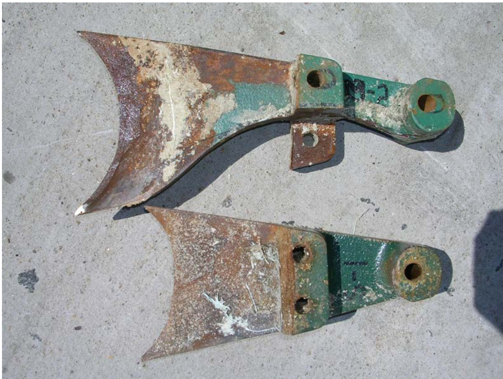
Figure 2 – A splitter with a reverse curve (top) lifts the groundline out of the hauler gradually in comparison to a straight-sided splitter (bottom).
