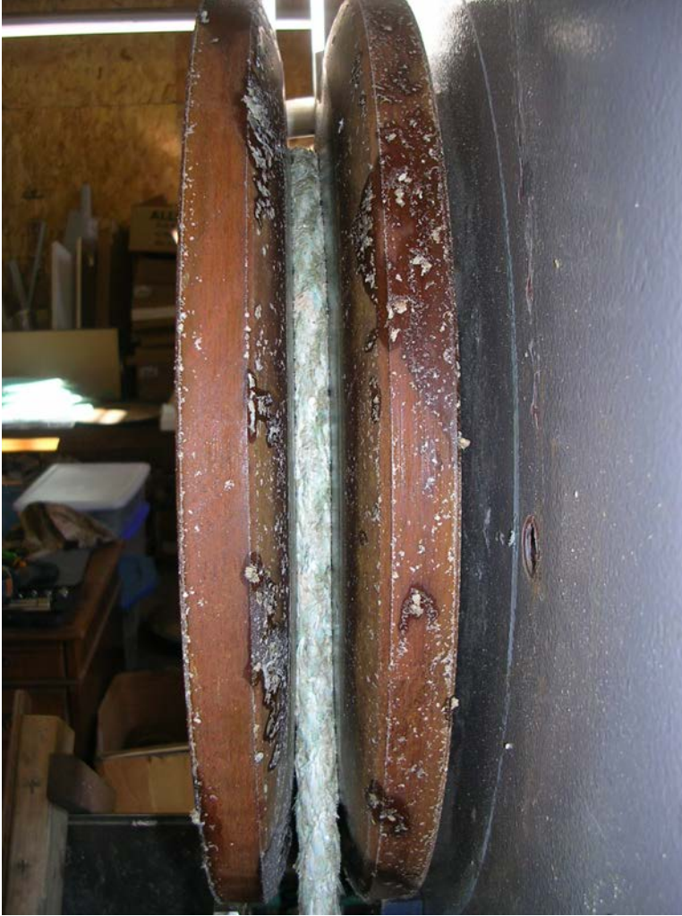
Figure 1 Lobster trap haulers work by wedging the pot warp between two steel discs. Higher tension in the line causes it to wedge more deeply into the V between the discs.
