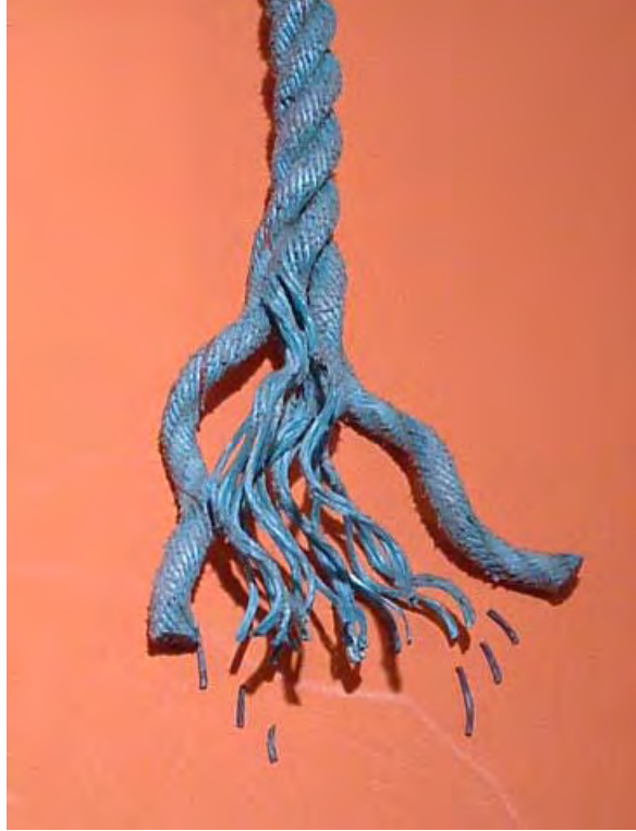
3-strand rope with 19 yarn ends per strand and lead core in center of each strand. Broken core segments seen in photo.
